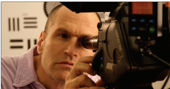
Al Collins ensures proper optical alignment using a Borescope, one of many diagnostic tools Fletcher's technicians use to maintain camera performance.
